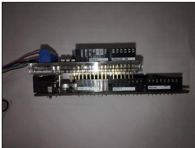
Figure 24 The motor shield attached on the top of Arduino 2560
